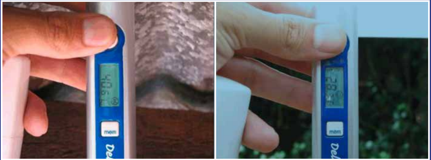
A temperature measurement under galvanized iron patio 40.6°C A temperature measurement under 4EVER SHEETING natural white 28.3°C
